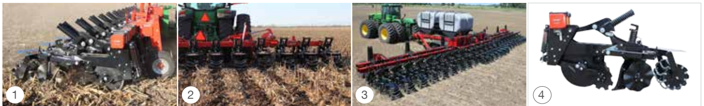
1. 3-Point Mounted / 2. Pull-Type / 3. 24-Row Strip-Till / 4. Individual ST-PRO™ Row Unit
