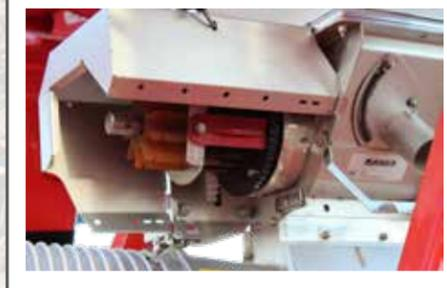
Fan driven hydraulically from tractor SCV. Speed can be adjusted to suit seed type by adjusting oil flow from tractor.
