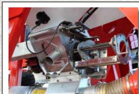
Electric drive metering unit with unique dual spline system. No components to add or remove when changing between small and large seed types or when switching between rates.
