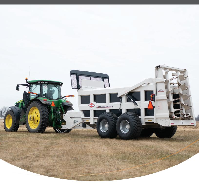
The new KUHN Knight HP 160 hydraulic push box spreader features the proven ProPush® design customers have come to love, in a higher capacity, commercial-duty package. The HP 160 with VertiSpread® vertical beaters is designed to haul and spread solid materials from dairies and feedlots, including gutter manure, yard scrapings, bedding pack and feedlot manure. The hydraulic push-type design means no apron chains, fewer moving parts and dependable service life.
