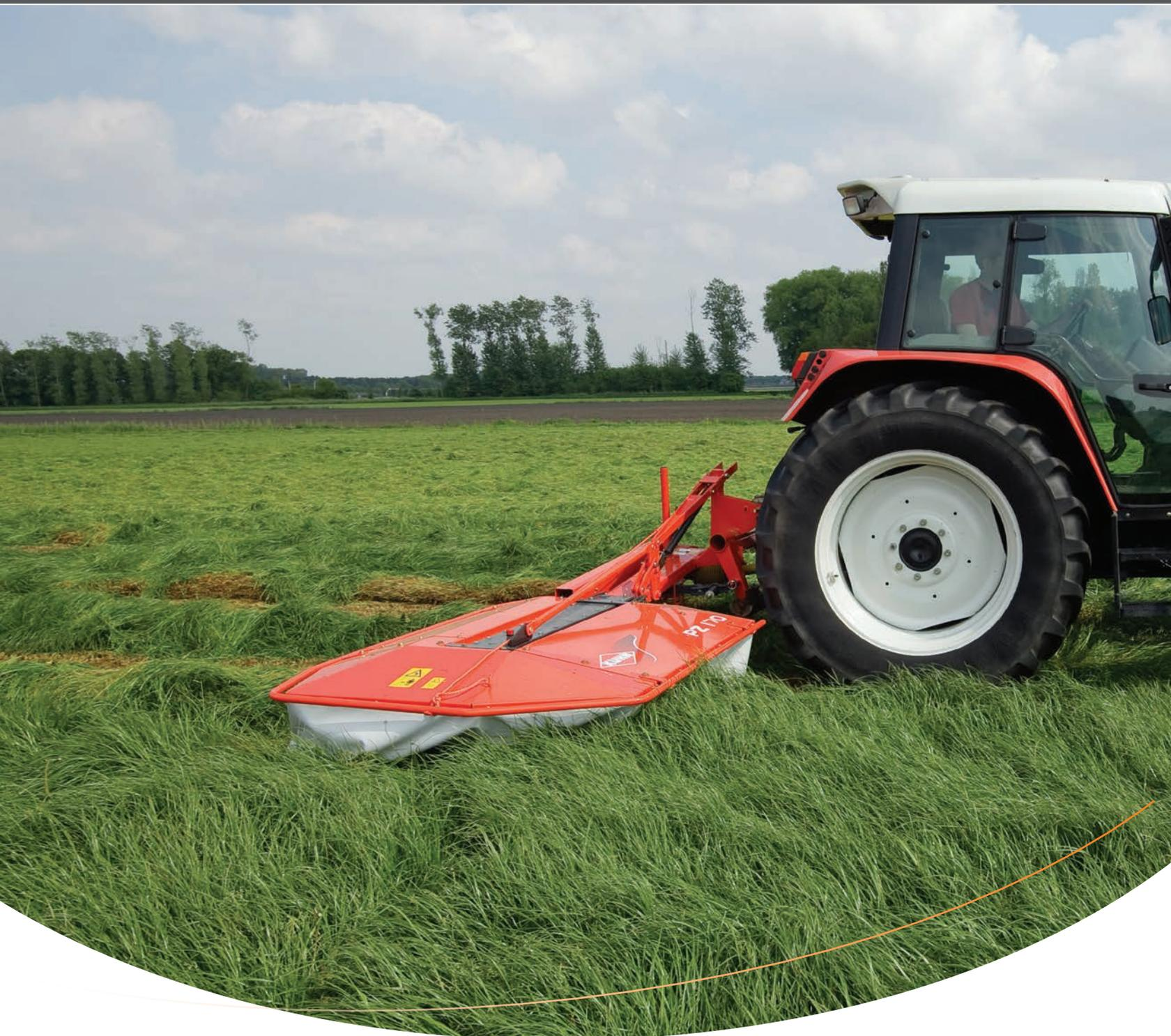
The 5'5" cutting width of the KUHN PZ 170 drum mower provides small-acreage landowners and hay producers with significantly improved capacity and productivity compared to sicklebar mowers. This drum mower easily cuts through tall, thick and tangled grasses with minimal horsepower required. Designed to be reliable and simple to operate, the PZ 170 builds on a legacy that goes back over 50 years to the introduction of the world's first drum mowers.
