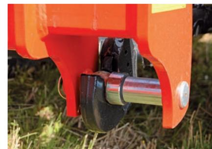
A wide range of hitch categories are available (Cat. 3, 4N, 4, Quick hitch 3 and 4N) to adapt to medium and high power tractors (135 to 360 hp).
