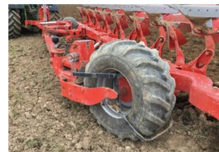
A large tire supported on both sides ensures stability in headland turns and provides a longer hub life. The 500/60-22.5 lug-type tire shown above is standard on the Multi-Leader XT and optional on the Vari-Leader models.
