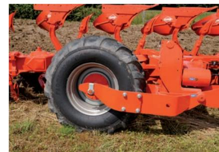
A stub axle mounted on tapered roller bearings makes this turning system incredibly reliable.
