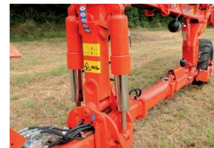
With two telescopic, single-acting cylinders, headland turns are jolt free. This also reduces stress on the tractor's lift arms allowing for optimum comfort during turns.
