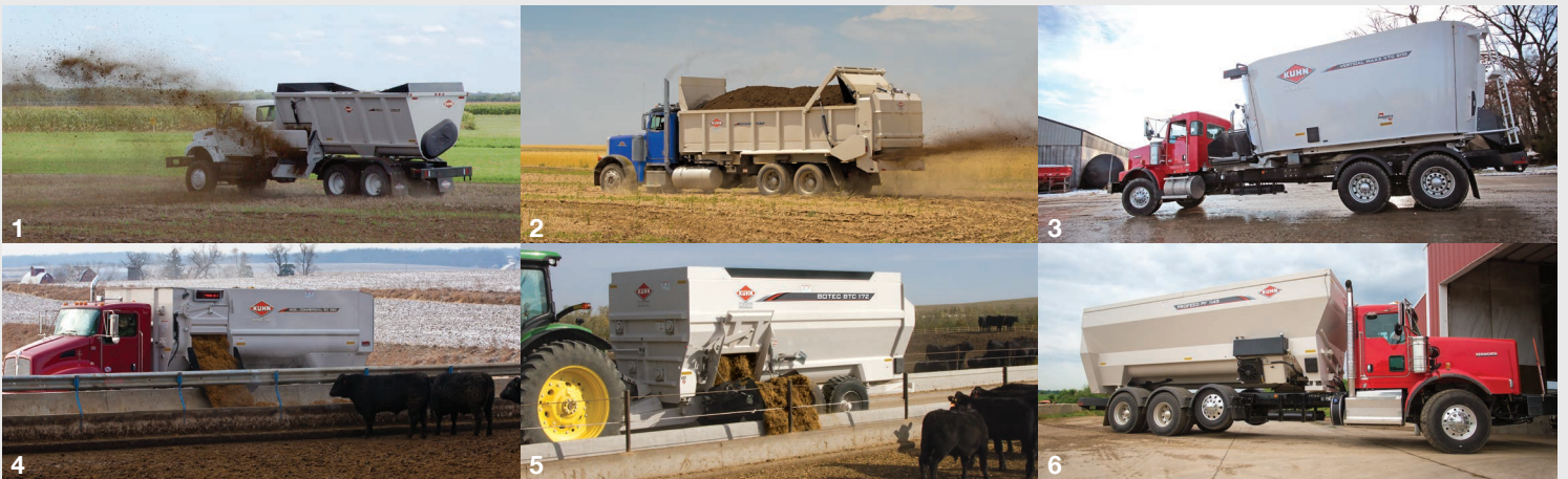
1. Side-Discharge Spreaders – 2. Apron Box Spreaders – 3. Vertical Twin-Auger Mixers – 4. Reel Mixers – 5. 4-Auger Mixers – 6. Delivery Boxes
